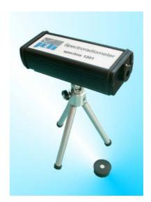
Pulsed sources are measured in illuminance mode using the diffusor cap. The instrument measures the cycletime of a pulsed source with an additional detector in the front face. The following spectral measurement will be synchronized with the measured lamp cycle. Radiometric and photometric values are indicated in exposure per puls.
